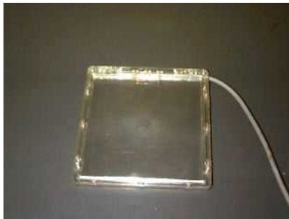
An exposure-area product detector used in radiography.
