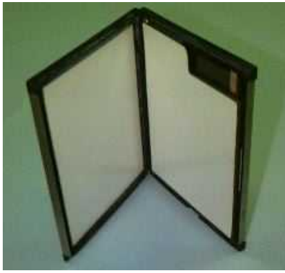
An X-ray cassette used in radiography.
