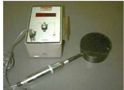
An exposure meter used in radiography.
