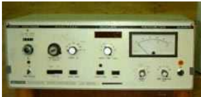
A single channel analyser.
