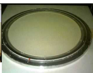
The NaI crystal of a gamma camera.
